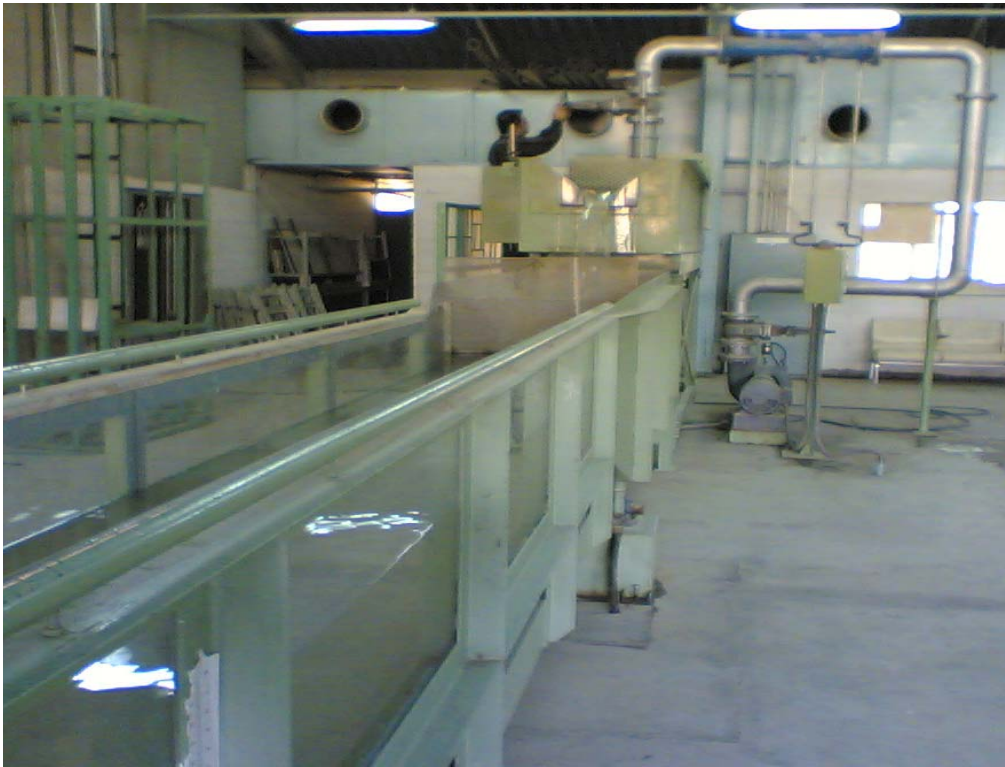
Plate 1. Photograph showing the laboratory horizontal channel with V-notched tank and dissipation tank.
