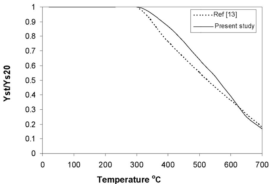
Figure 6. Variation of steel yield strength with temperature rise.
