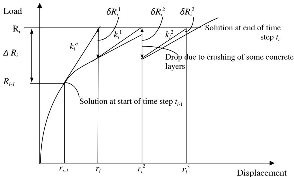
Figure 7. Solution of time dependent nonlinear equilibrium equation.
