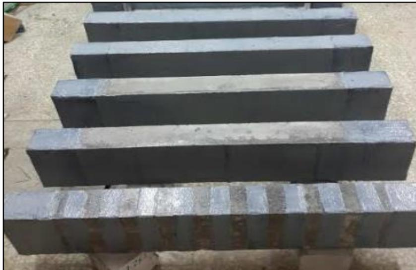
Figure (5): Strengthened beams
