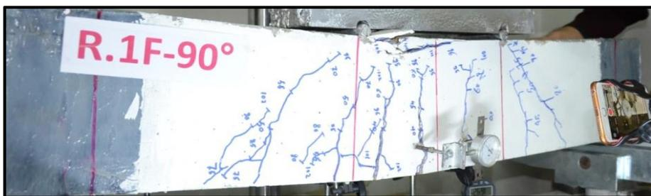
Figure (17): Crack pattern of beam (R.1F-90°)
