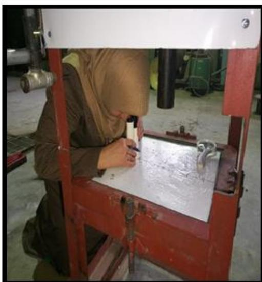
**a) Crack width measuring by Portable Microscope.**
