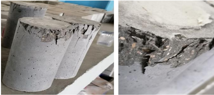
Figure 6. Damage and failure mode after compressive strength test for the optimized mix
