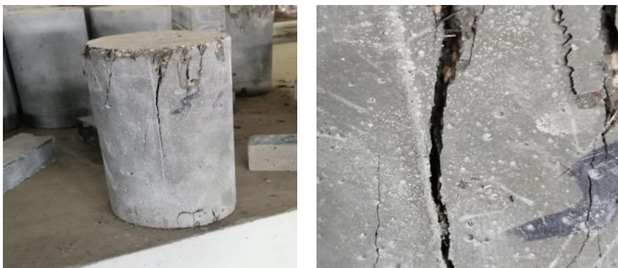
Figure 8. Damage and failure mode after tensile strength test for the optimized mix
