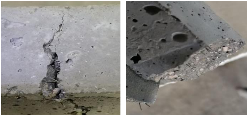
Figure 7. Damage and failure mode after flexural strength test for the optimized mix
