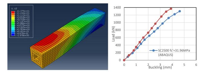
Fig. (9-c) Concrete failure under eccentricity (SC3H)
