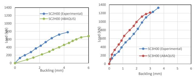
Fig. (11) Load-buckling curve (SC3H00)
