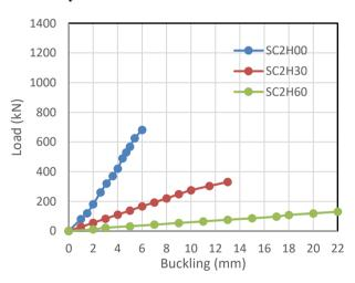
Fig. (13-c) Load-buckling curve (SC2H) for different eccentricity
