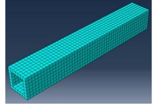
Fig. (1) Meshing of steel tube.
