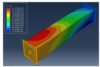
Fig. (9-a) Column failure under eccentricity (SC3H)
