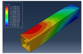
Fig. (9-b) Steel tube failure under eccentricity (SC3H)
